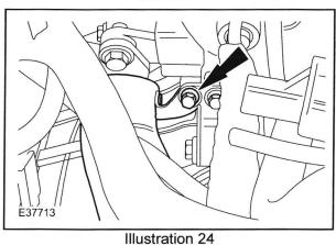
18. Remove EGR transfer pipe to EGR valve securing screws (see Illustration 25).
