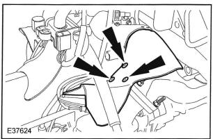
17. Remove EGR transfer pipe heat shield securing screw and remove heat shield from vehicle (see Illustration 24).
