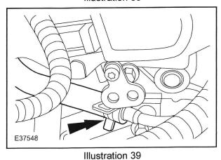
44. Re-install right-hand camshaft position sensor electrical harness (see Illustration 40).
