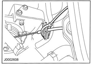
11. Reposition the accelerator pulley to the full throttle position and disconnect accelerator inner cable (see Illustration 18).
