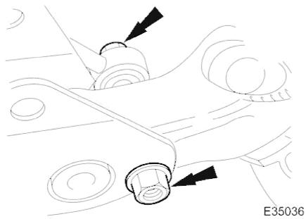
9. Align stabilizer bar link rod with lower wishbone, install nut and bolt and tighten to 39-55Nm.
