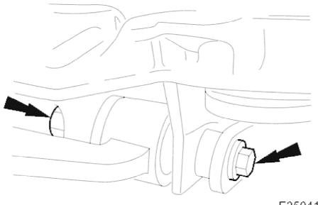
E35041 9. Remove nut and bolt securing lower wishbone front arm to cross-beam.
