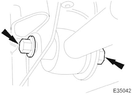
7. Tighten wishbone rear arm pivot nut and bolt to 113-153Nm.
