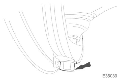
4. Install nut securing lower ball joint to vertical link and tighten to 60-80Nm.
