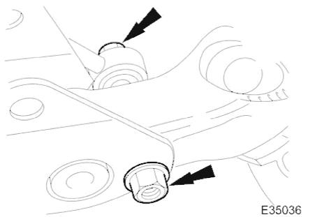
3. Remove nut and bolt securing stabilizer bar link-rod to lower wishbone.
