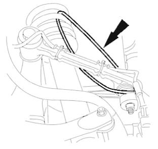
6. Remove wire temporarily securing vertical link to road spring.
