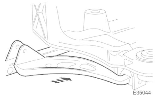
1. Position lower wishbone on suspension cross-beam and vertical link.
