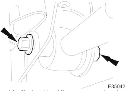
2. Install but do not tighten wishbone rear arm to cross beam pivot nut and bolt.
