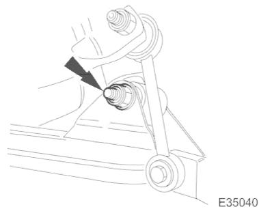
5. Align lower end of shock absorber with wishbone, install nut and bolt and tighten to 60-80Nm.
