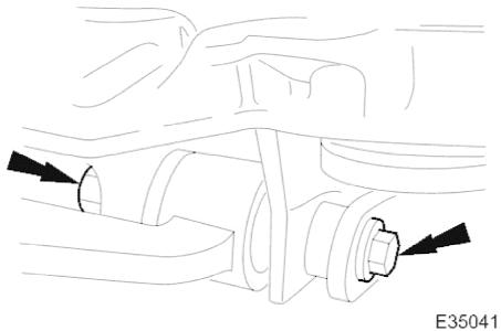
8. Tighten wishbone front arm pivot nut and bolt to 113-153Nm.
