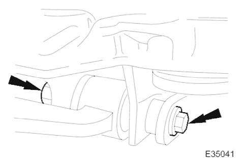
3. Install but do not tighten wishbone front arm to cross beam pivot nut and bolt.
