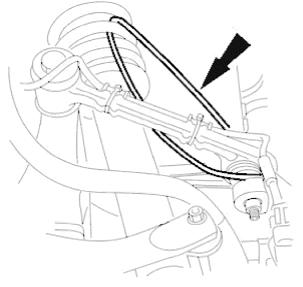
4. To prevent damage to upper ball joint, secure vertical link to road spring using strong wire.
