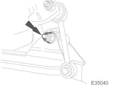
8. Remove shock absorber lower nut and bolt.
