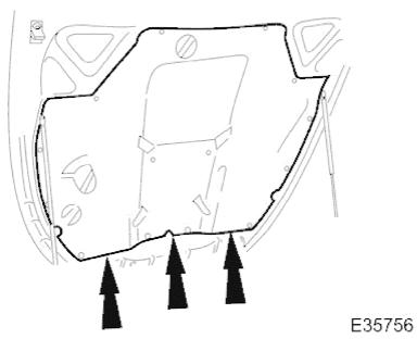
7. Commencing at bottom, remove retainers from insulation pad.
