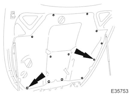
6. Slacken and remove expander screws from hood insulation pad retainers.
