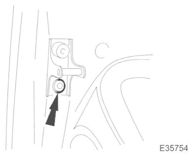
9. Slacken and remove bolts securing striker/buffer assemblies to hood and remove assemblies.
