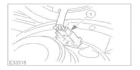
5. Disconnect and remove the speaker.1. Support the speaker, disconnect the multi-plug and remove the speaker.
