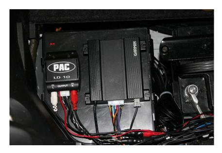
A convenient source of power in the trunk is the trunk accessory connector, which is an unused three pin connector adjacent to the battery which provides Ignition switch power, battery +12v and ground. Be sure to check whether trunk fuse box relay number 6 and fuse number 11 are present...you may need to add them. The relay is a standard automotive single pole type available from any auto parts store.
