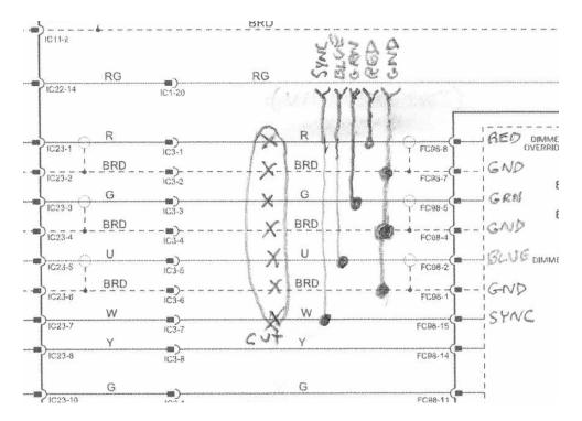
Also, before connecting the converter, definitely follow the advice in the instructions and test mate the two molex connectors that are spliced in the circuit to make sure your splices are done property.
