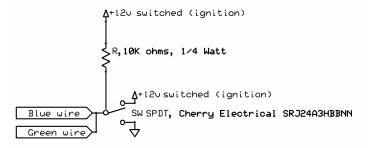
The three positions of the switch are then video 1 (center to +12), original nav. video (center off) and video 2 (center to ground).
