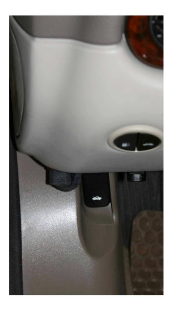
Note also in the photo the optical sensor for the remote to the right of the parking brake release. The optical sensor should be mounting location is more of a personal preference, but it should not face directly up and it should be roughly line of sight with your hand when you operate the remote.
