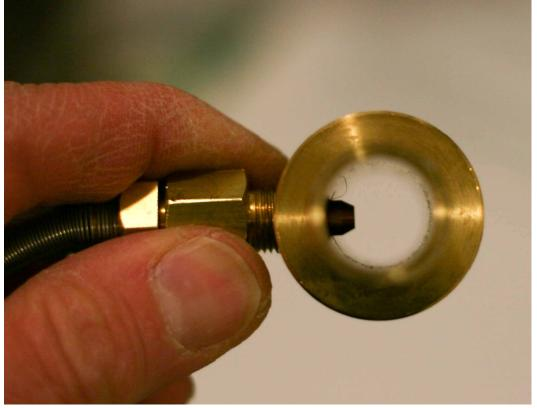
Use 2-3 turns of Teflon tape sealant on each connection.
