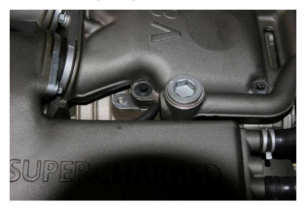
The fuel pressure regulator is under the right intake charge cooler, in the rear, and is accessible by just removing the intake pipe. Use fresh new vacuum hose when you make these connections. Also, according to the HKS instructions, the hose feeding the pressure sensor should be fitted with the inline air filter specified in the materials list to prevent contamination.
