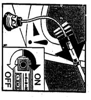
Switch radio off for a moment and then on. This should fully extend the telescope and toothed plastic wire. Do not extend the telescope by hand. The electronic control limits duration of operation at approximately 12 seconds.
