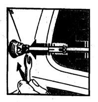
Switch radio off and drop the plastic wire into the mounting hole until teeth are engaged by the drive. If the plastic wire is not pulled into the drive, the drive has not engaged the teeth. If this occurs, switch radio off and on and turn plastic wire up to 180 degrees until teeth on wire connect with the drive. As the plastic wire is drawn in, gently push the telescope's tubes into the housing. Then insert the threaded bushing.
