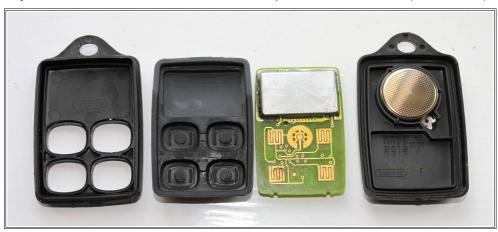
8) Notice the dirt and residue on the printed circuit board and inside the rubber surround. This needs to be cleaned off.
