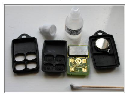
13) Now reassemble the key fob, place the electrics back into its rubber surround, place the surround back into the front half of the plastic fob casing.
