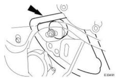
13. Move glass regulator stop to abut quadrant and tighten adjuster bolt.
