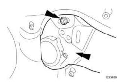
${\bf 11.}$  Remove tape from access hole in PVC secondary water shedder and slacken glass regulator stop adjuster bolt.
