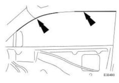
12. Motor door glass further up until the horizontal datum line aligns with the upper seal.
