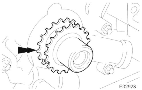
3. Remove the sprocket from the crankshaft. To remove the Bank 2 sprocket, the Bank 1 sprocket must be removed first.
