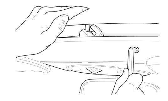
In the event of latch failure when the top is raised, a visual warning will illuminate on instrument panel. In such an emergency, the top must be manually positioned using a center pull down facility, then latched using a key stowed alongside the top operating pump. To manually operate the latch, the key is inserted in the recess in the windscreen header, turned clockwise to ensure the latch is fully released, then turned counter-clockwise to lock.
