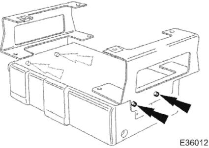
7. Withdraw autochanger/mounting bracket assembly from trunk and remove four bolts securing autochanger to bracket.
