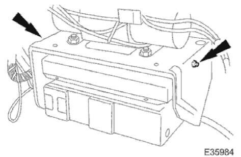
6. Remove side bolts securing autochanger mounting bracket to outer mounting bracket
