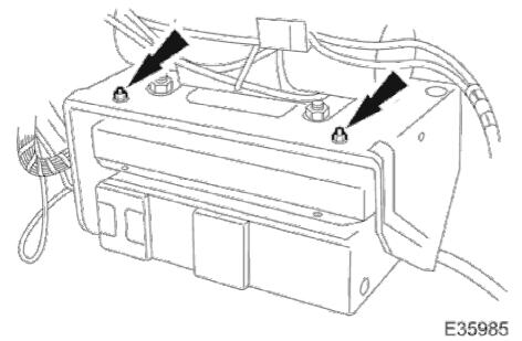
5. Remove upper bolts securing autochanger mounting bracket to outer mounting bracket.
