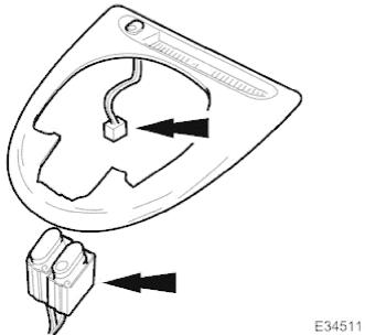
5. Position the veneer panel for access and disconnect the panel switch multiplugs.
