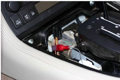
11. Using a red T-Tap, connect the BROWN wire from the Pulse Timer to the Green-Black WINDOW-UP relay wire. See photo below and drawing at the end of this section. (Note: there are 2 Green-Black wires in this cable at this connector RH12, make sure you use the one that is third wire from the bottom of the connector – ask me how I know!)
