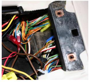
12. Using a red T-Tap, connect the RED wire from the Pulse Timer and a new red wire to connect to the relay to the Brown-Red B+ wire at the telephone connector on the left side of the console. See photo below and drawing at the end of this section.
