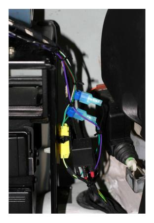
5. Using a red T-Tap, connect the BROWN wire from the Pulse Timer to the Green-Blue WINDOW-DOWN relay wire. See photo below and drawing at the end of this section.
