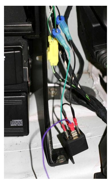
4. Mount the relay to the yellow pump valve connector on the right side of the audio rack with a tie wrap. See photo below:
