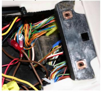
6. Using a red T-Tap, connect the RED wire from the Pulse Timer to the Brown-Red B+ wire at the telephone connector on the left side of the console. See photo below and drawing at the end of this section.
