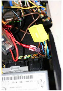
13. Complete <u>all remaining connections</u> of the relay and pulse timer in the right rear of the console as shown in the drawing at the end of this section (this can be accomplished with the console in place (though it might be a bit easier with the console removed). The relay wiring is shown in the photo below:
