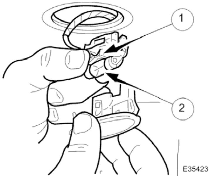
2. Remove the bulb from the roof lamp.
